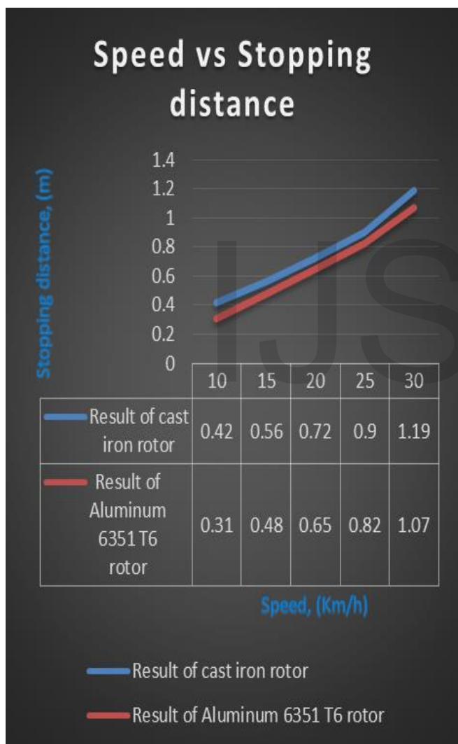
FIGURE III. COMPARISON OF SPEED VS STOPPING DISTANCE BETWEEN CAST IRON AND ALUMINUM 6351 T6 ROTOR
